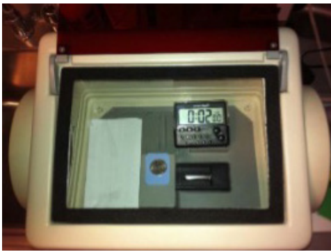
Figure 1 – Intraoral Fog Test Set-up in a Glove box
